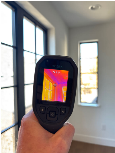
NORMAL THERMAL READINGS - INTERIOR
